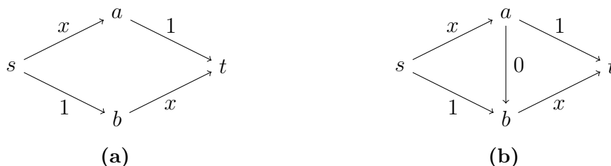
Figure 3.2: Braess paradox for cost reductions. The network in 3.2b features a low cost edge not present in 3.2a, but the cost on its equilibrium path is higher.
